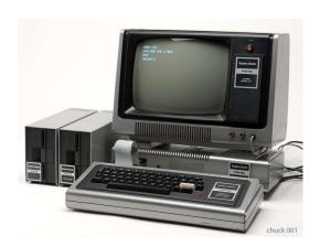
This \$1000 business machine was equipped with an 8K ram motherboard and 2 5 1/4" external floppy disks, each with 84k of memory and access to a printer. The ability to type letters without having to use a typewriter and the automatic tallying of accounting ledger columns was worth every penny of its cost.
